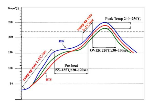
ramp up rate(30~150  $^{\circ}$ C): 1.0~2.0  $^{\circ}$ C/sec pre-heating time(155~185  $^{\circ}$ C): 30~120 sec time period above 220  $^{\circ}$ C: 30~100 sec ramp up rate during reflow: 1.0~2.0  $^{\circ}$ C/sec peak temperature: 240~250  $^{\circ}$ C ramp down rate during cooling: 1.0~6.0  $^{\circ}$ C/sec
